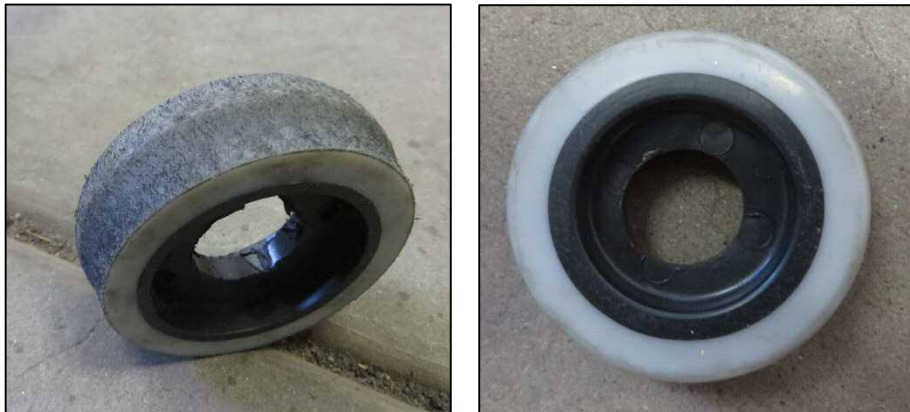
Figure 7- Worn Wheel vs. New Wheel
